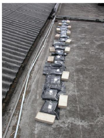
**Figure 3. Plastic bags on the balcony of the laboratory exposed to sun light with bricks holding them because of the wind.**
