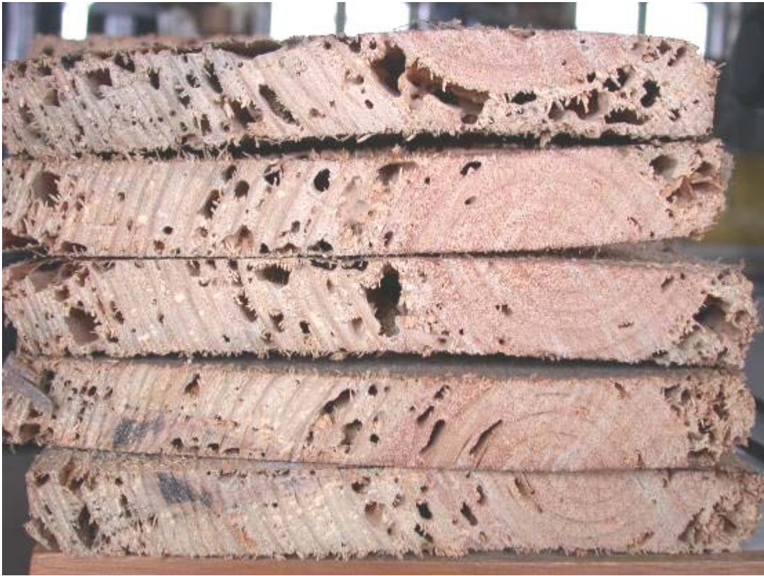
Figure 3. Consumption of sapwood by Cryptotermes brevis .
